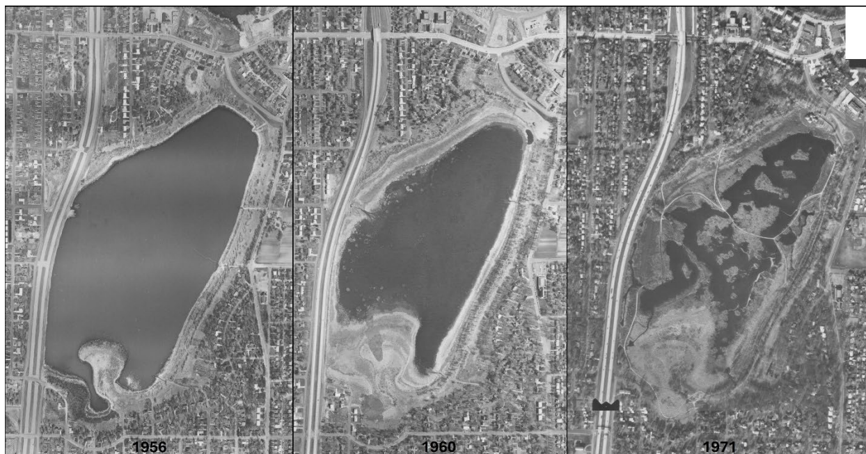
Figure 13. Aerial images of Wood Lake in 1956, 1960, and 1971 showing water level reduction and increase in exposed shoreline and vegetated shallow wetlands (CITE MHAPO).
